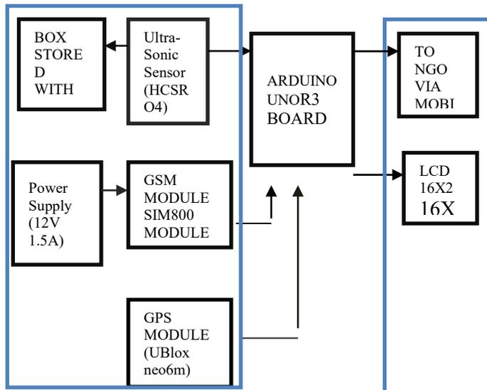
Fig. 1. Block diagram showing the hardware components used
