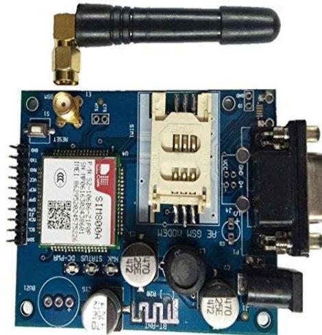
Figure 3: GSM module (SIM 800A)
