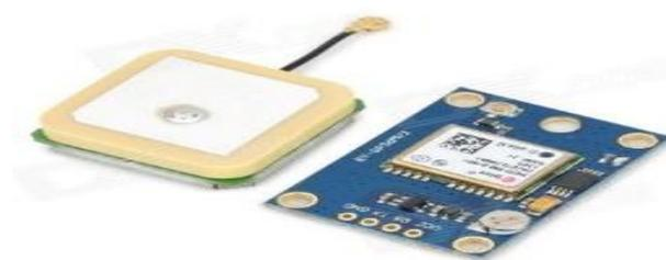
Figure 4: U-BLOX NEO-6M GPS Module
