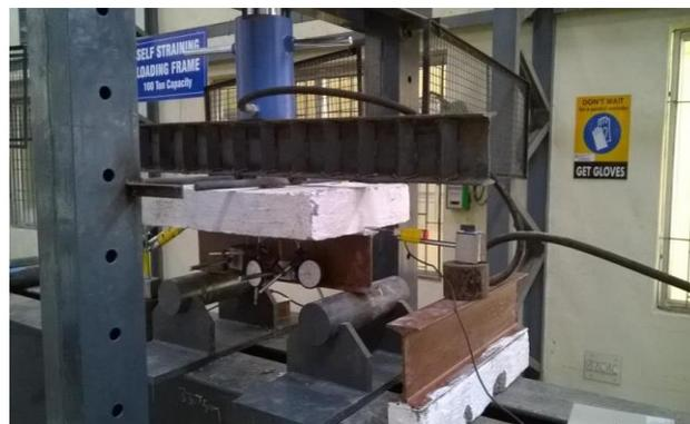
The following are the readings of the shear connector welded composite beam (I section with concrete slab) is as shown in tabular and the failure load of specimen is as shown in fig given below with the results.
