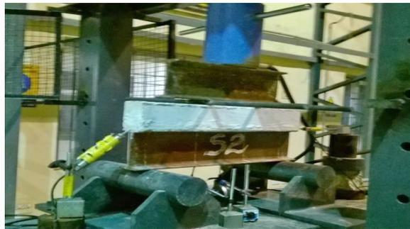
The following are the readings of the shear connector welded composite beam (I section with concrete beam) is as shown in fig. and the failure load of specimen with the results.
