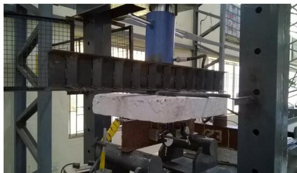
The following are the readings of the shear connector welded composite beam (I section with concrete slab) and the failure load of specimen is as shown in abovefig, with the results.
