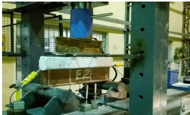
The following are the readings of the shear connector welded composite beam (I section with concrete beam) and the failure load of specimen is as shown in fig with the results.,
