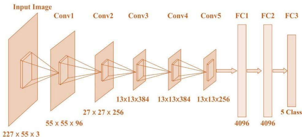
Fig. 1 Structure of AlexNet
