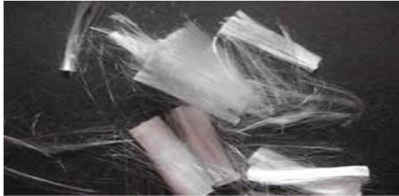
**Figure: Polypropylene fibre**
