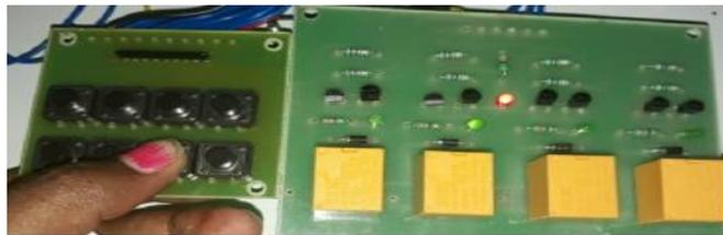
Figure 9 Pressing the push button 2 to pick the child
