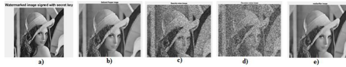
Fig 4 a) Watermarked image b) Salt and Pepper Noise c) Speckle Noise d) Gaussian Noise e) Median Filter.
