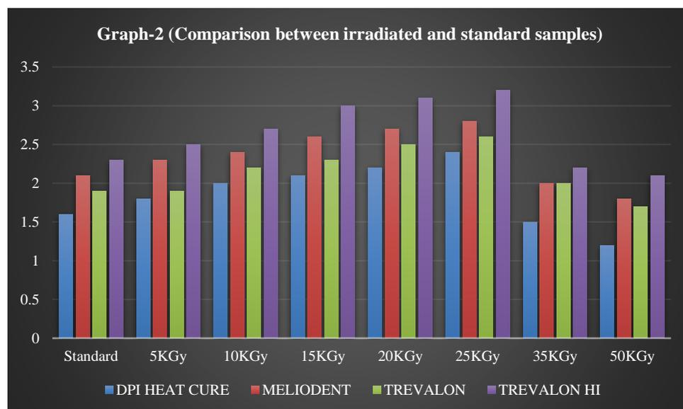
Fracture toughness (the ability of a material to resist crack propagation,) is an important property for denture base resins, preventing or reducing the incidence of denture fracture, thus decreasing patient discomfort and reducing the number of appointments for denture replacement or repair.
