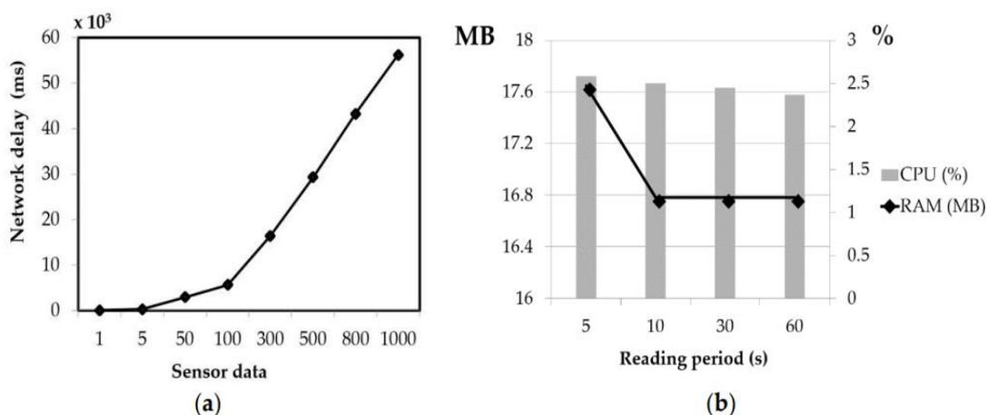
FIGURE 7: IoT-based sensor system’s (a) network delay and (b) CPU and memory usage
