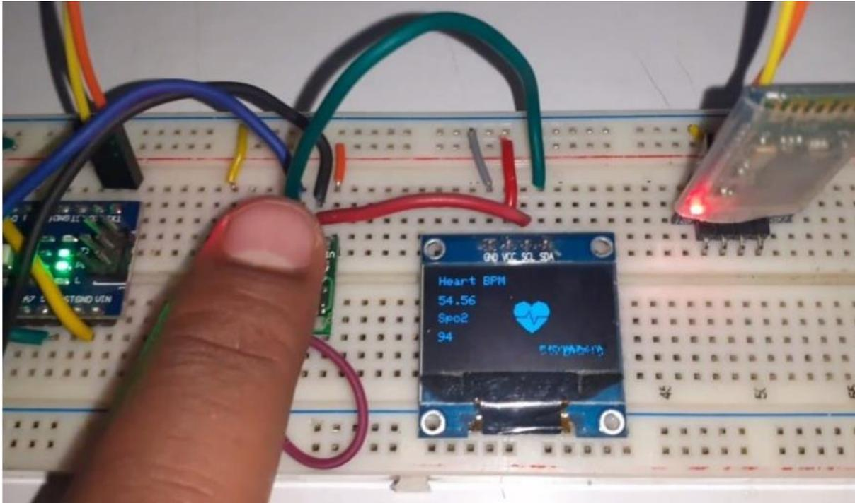
FIGURE 4:INTERFACING OF PULSEOXIMETER WITH ARDUINO NANO
