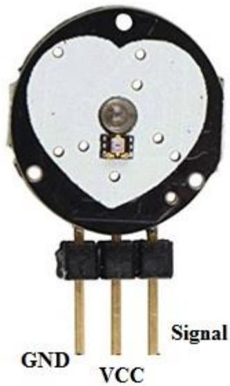
Figure 3: Heart Rate Sensor
