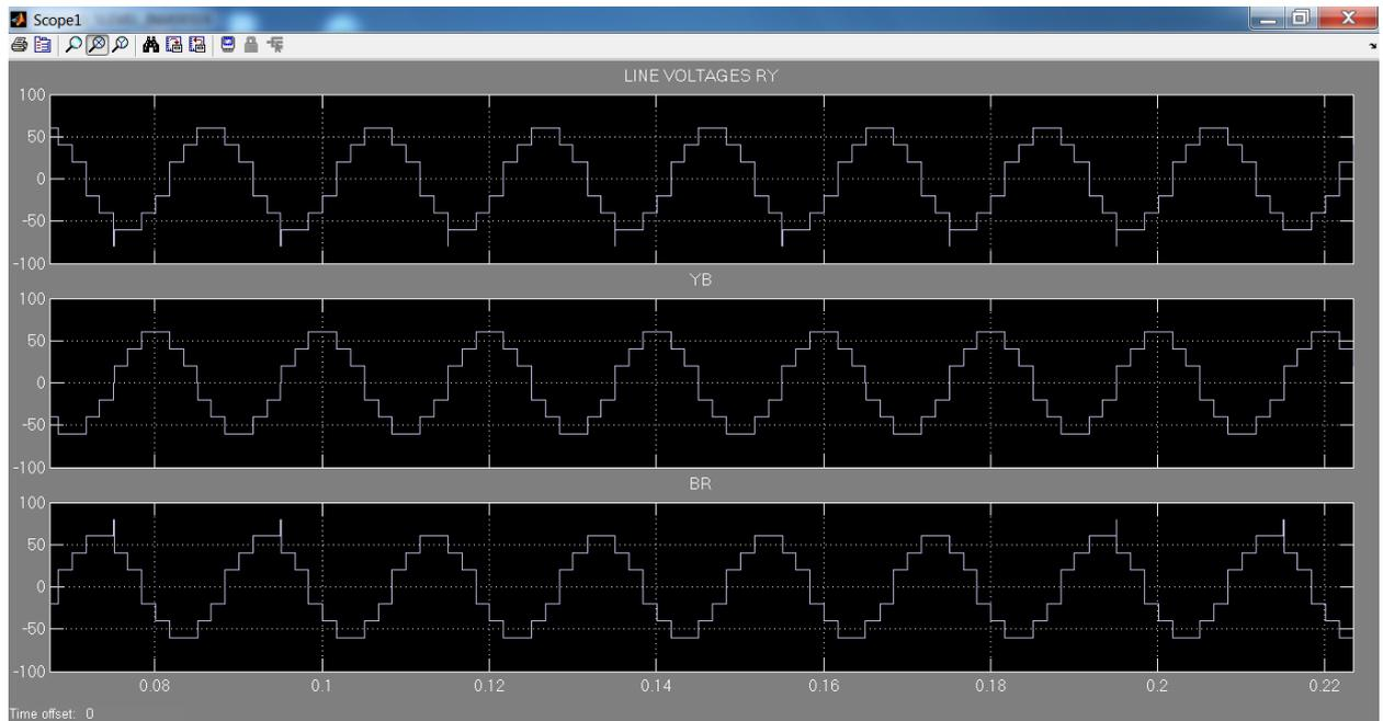
Figure 7: MATLAB Simulink graph for three-phase 5-level cascaded H-bridge inverter line voltage output.
