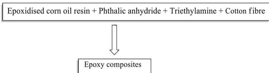
**Scheme 4. Formation of cotton fibre reinforced composites**
