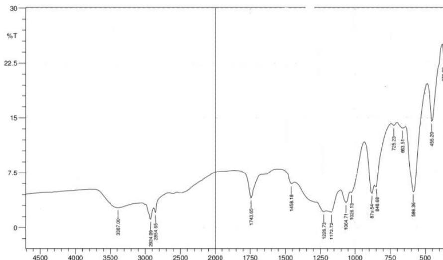
**Figure 1. FT-IR spectrum of Epoxidised corn oil resin**
