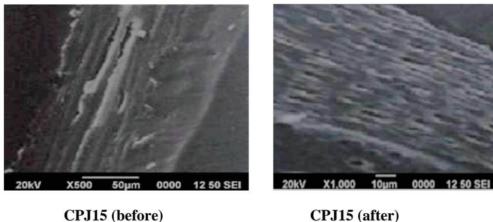
**Figure 2. SEM images for the biodegradable composites CPJ10 and CPJ15 before and after soil burial test**
