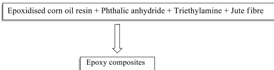
**Scheme 3. Formation of jute fibre reinforced composites**
