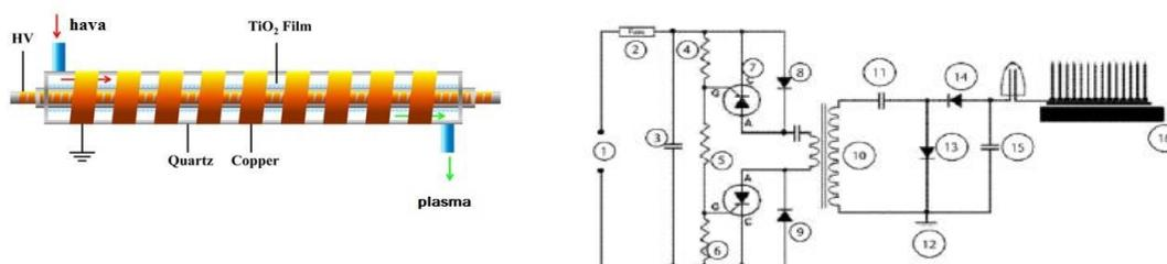
**Fig. 1.** Schematic of the nano- plasma air purification device.
