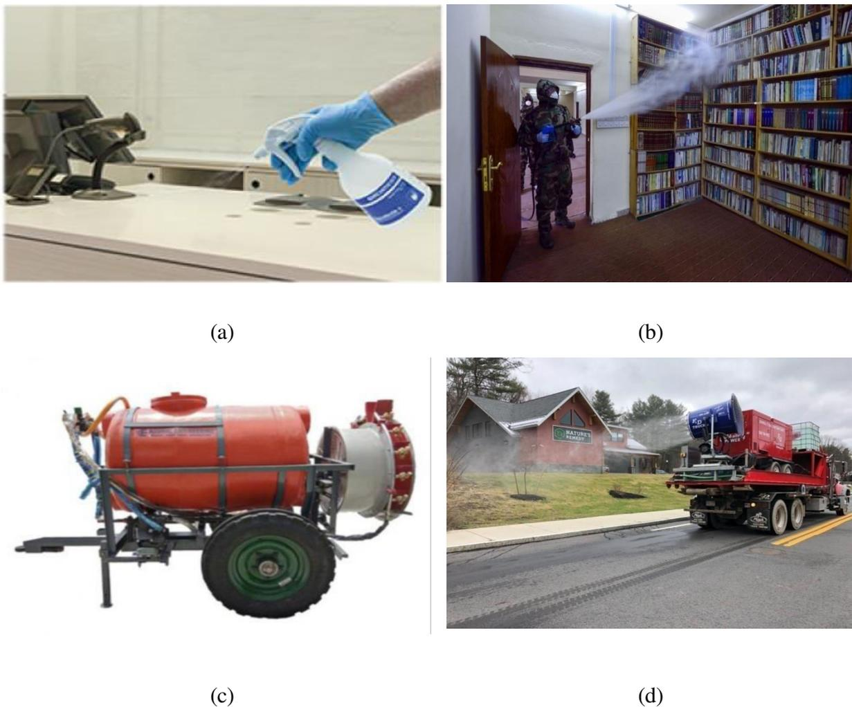
Figure 3: Various spraying equipment, a) Hand sprayer; b) Fogger used in library; c) Mist cannons; d) Air assisted sprayer
