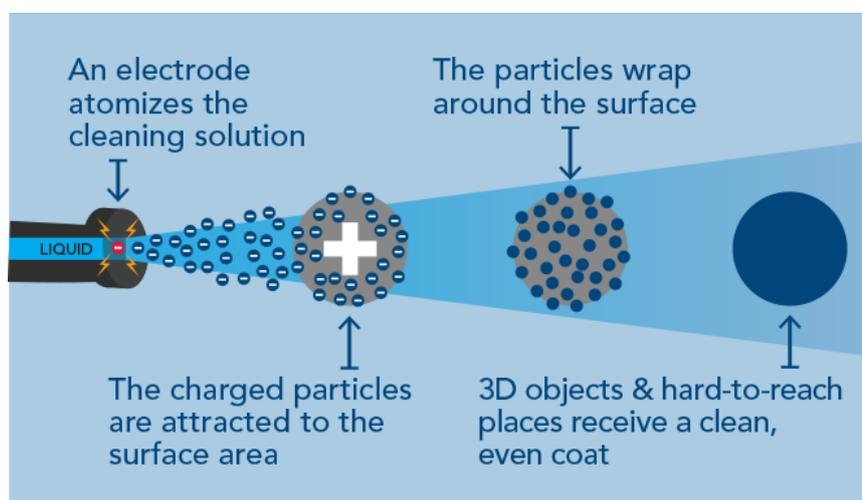
Figure 5: Principle of electrostatic spraying (CCC, 2020)
