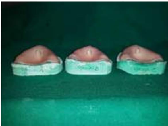
**Figure 12 finished denture bases**
