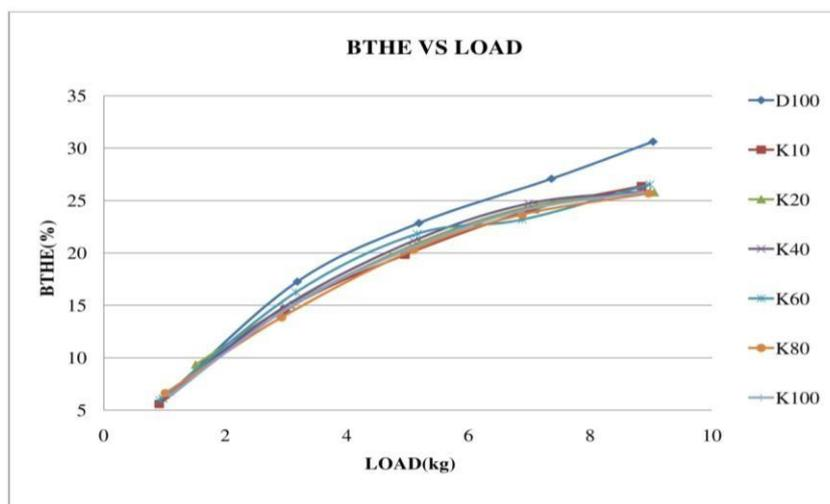
**Fig. 5:** Variations of Brake thermal efficiency with Load
