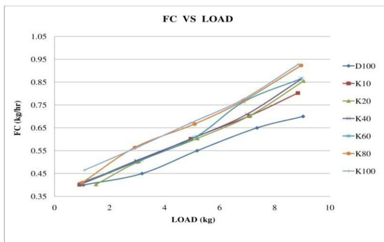
**Fig. 2:** Variations of Fuel consumption with Load
