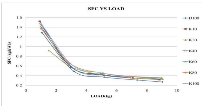
**Fig. 3:** Variations of Specific fuel consumption with Load
