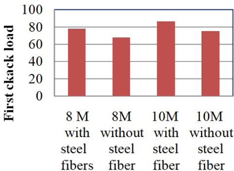
Mix Id Cracking Loads
