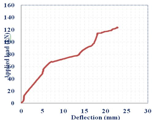
Load vs. deflection curve without steel fibers 10
