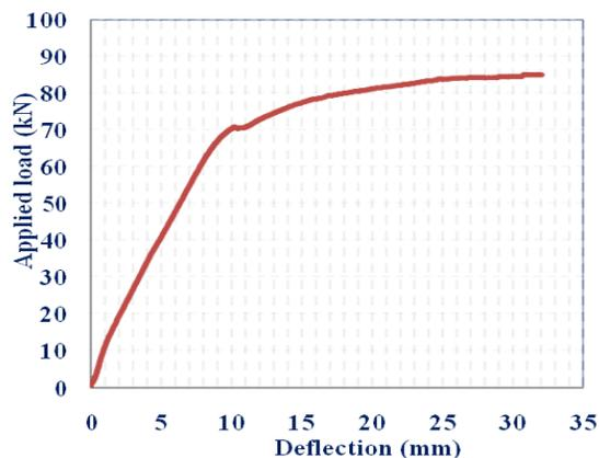
Load vs. deflection curve with steel fibers 10M
