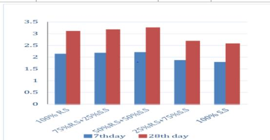
**Figure 5. Concrete STS with normal sand taken from river & sea**
