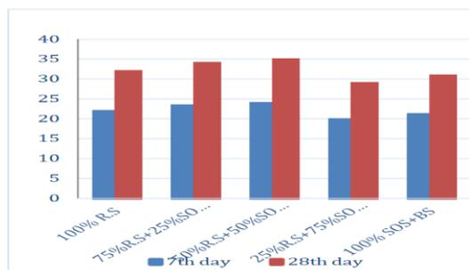
**Figure 8. Concrete CS with normal sand taken from river & boiled soaked sea**
