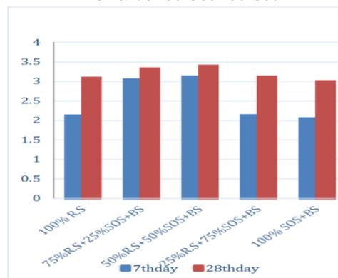
**Figure 9. Concrete STS with normal sand taken from river & boiled soaked sea**
