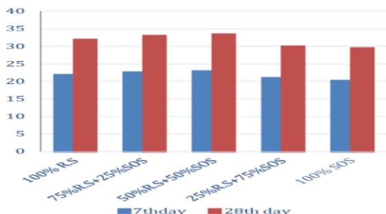
**Figure 6. concrete CS with normal sand taken from river & soaked sea**
