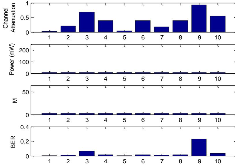
Figure 6: Channel attenuation, power, modulation and BER in low power mode using GWO
