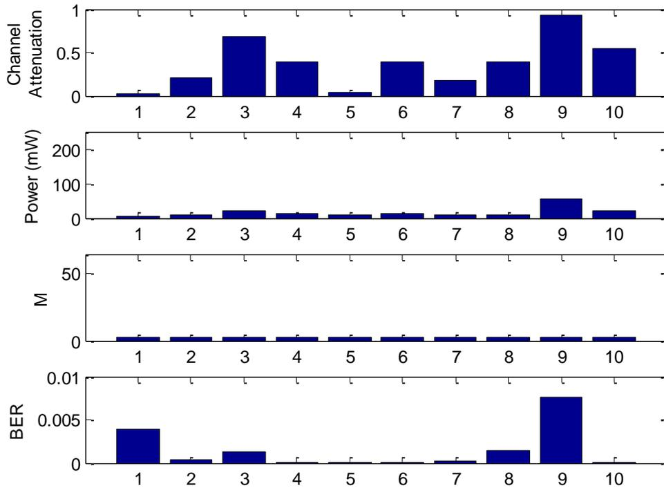
Figure 9: Channel attenuation, power, modulation and BER in balanced mode using GWO
