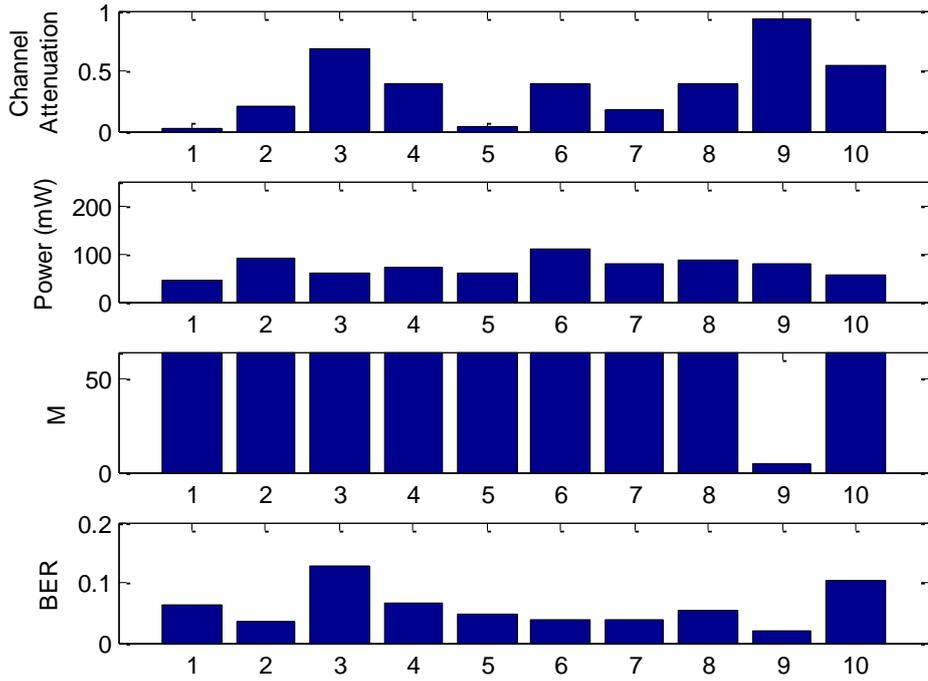
Figure 8: Channel attenuation, power, modulation and BER in multimedia mode using GWO
