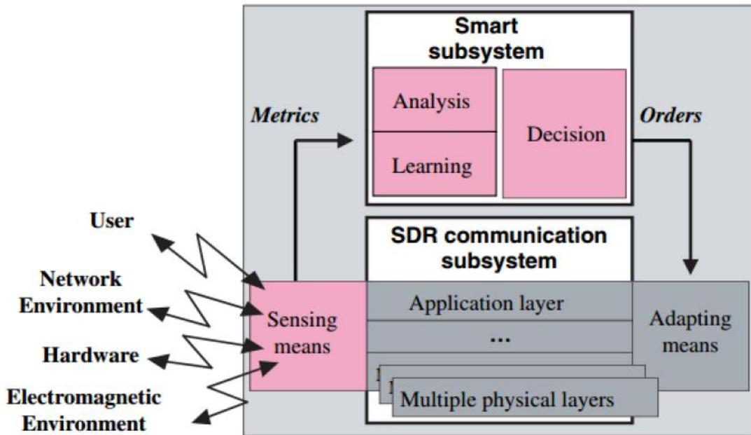
Figure 1: Synoptic diagram of a cognitive radio engine [12]
