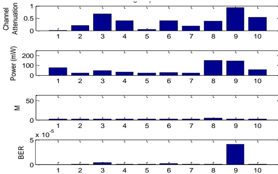
Figure 7: Channel attenuation, power, modulation and BER in emergency mode using GWO
