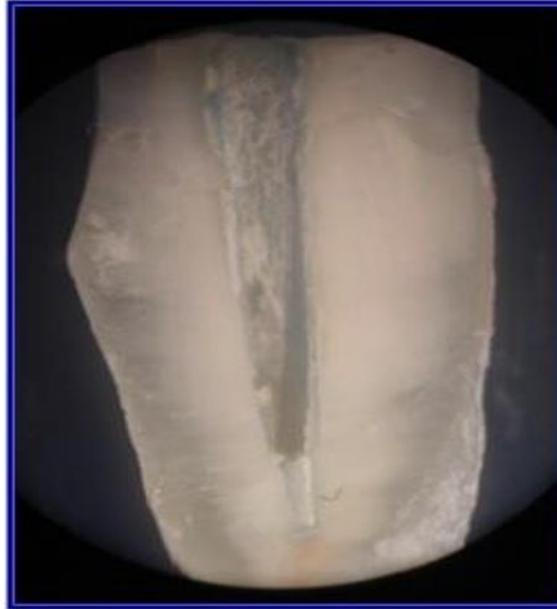
**Figure 4: Split specimen from the kodex twist drill/ parapost removal drill kit group demonstrating presence of post remnants in the cervical, middle and apical thirds**
