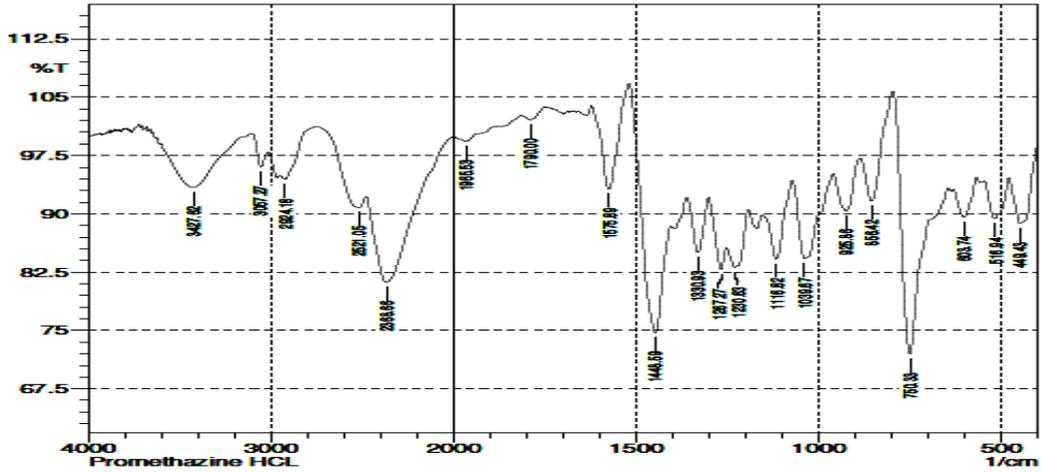
Figure 2: IR spectra of Promethazine HCL
