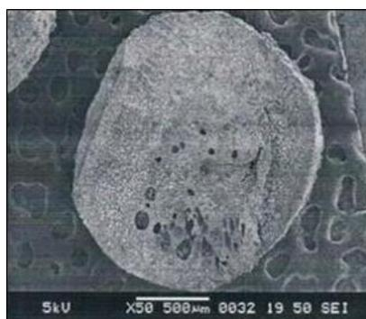
**Fig 4:** SEM-3 shows cross section view of microspheres at X50
