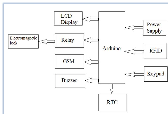
**Fig.1. Functional block diagram of the proposed system**
