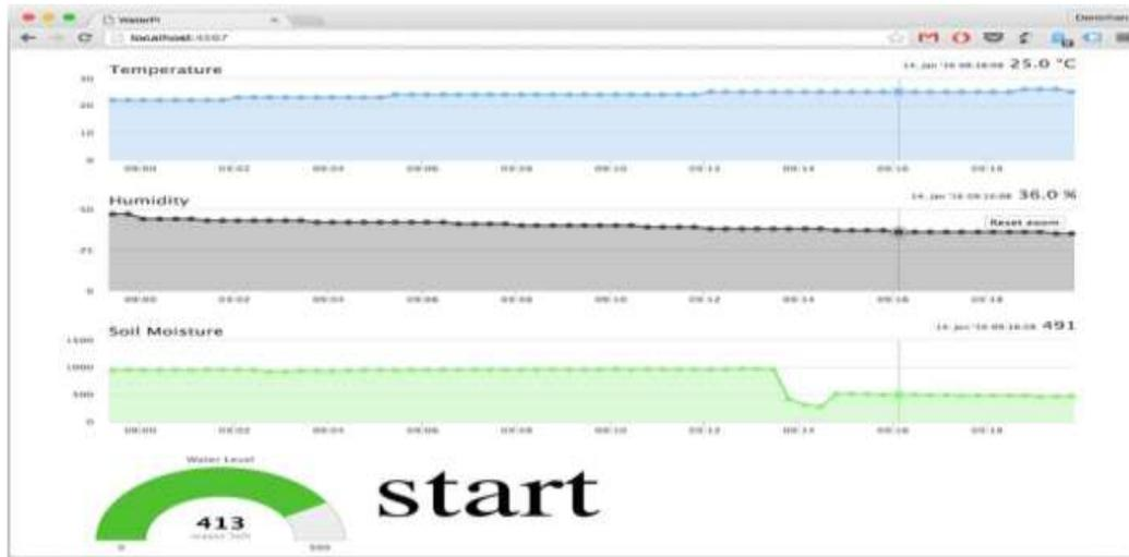
Figure 2: Web interface of the Remote plant watering and monitoring system based on IoT
