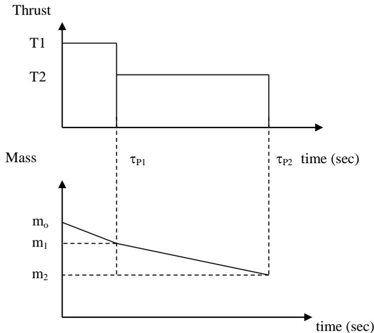
Fig. 1 Thrust and Mass Profiles
