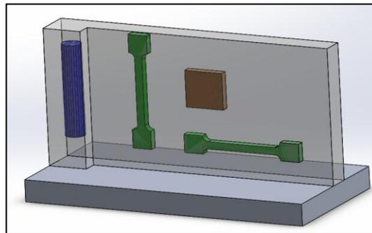
Figure3: CAD designs of specimens
