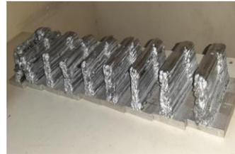
(b): Total of Nine Specimens prepared using WAAM
