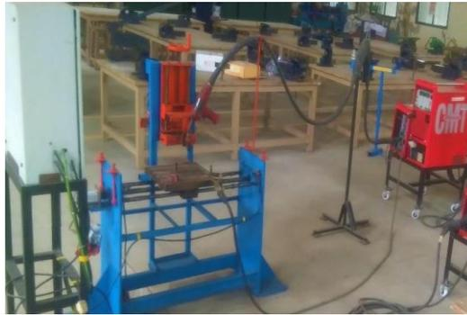
Figure1: Wire Arc Additive Manufacturing Apparatus
