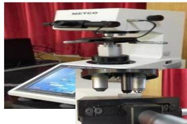
(b): Micro-Vickers hardness tester (with Macro view of diamond indenter and specimen)
