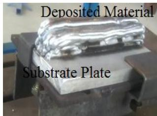
(a): Specimen Preparation on Substrate Plate
