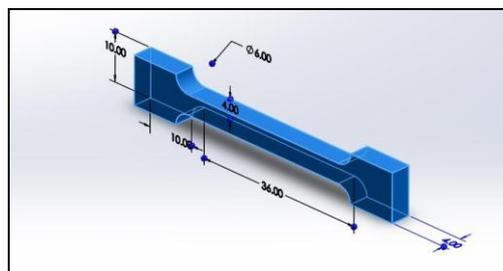
Figure4: Tensile test specimen as per ASTM standards
