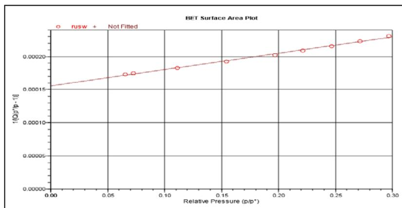
Figure (9): The surface area of the graphene prepared by BET method
