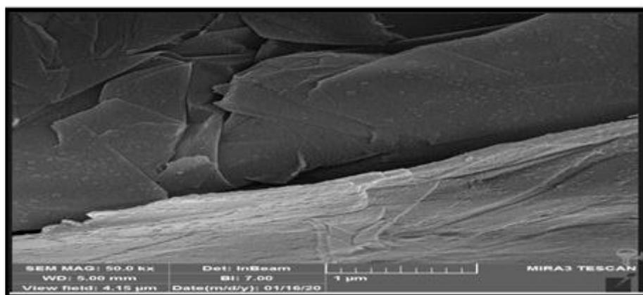
Figure (6): Image of a scanning electron microscope of reduced graphene oxide at 1µm scale
