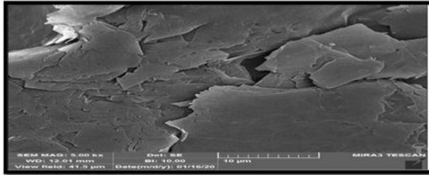
Figure (7) Image of a scanning electron microscope of 10µm reduced graphene oxide.
