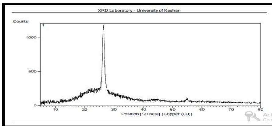
**Figure (5) X-ray diffraction spectrum of reduced graphene oxide**
