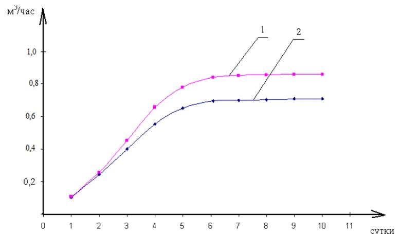
**Figure 2. The results of experimental studies on the output of biogas with various substrates: 1 - chicken droppings, 2 - cattle manure (cattle) in the period May**
