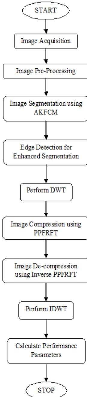
**Figure-1: Diagram of Proposed Work**
