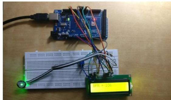
Fig 6: Mapping of Arduino with SEN11574(when finger is on the sensor)
