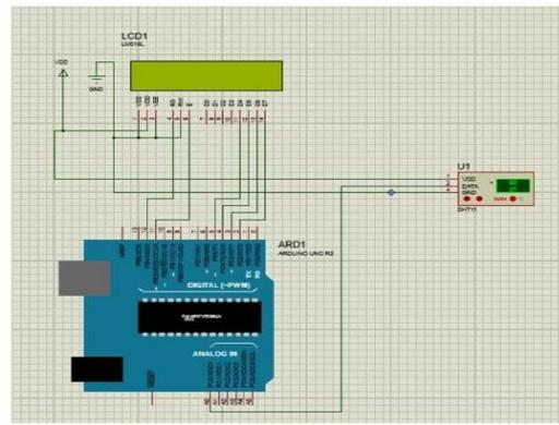
Fig 3: Interfacing of Arduino mega with 16X2 LCD
