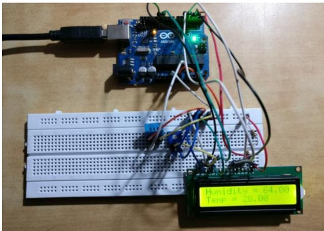
Fig 5: Mapping of Arduino with DHT11 and 16X2 LCD
