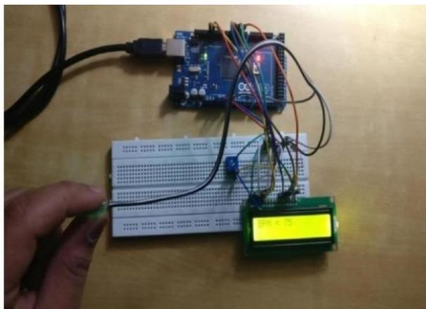
Fig 7: Mapping of Arduino with SEN11574 (when finger is not on the sensor)
