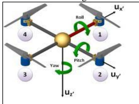
Fig.3 Common degrees of freedom of quadcopter
