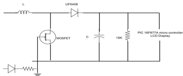
The Boost converter system for the above block diagram is as shown in figure 26 and the final block of Piezo electric generator is as shown in below figure 15.
