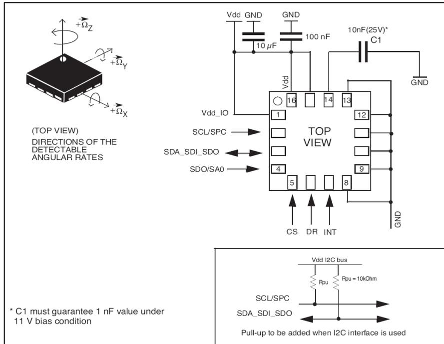
Fig.7 L3GD20 electrical connections and external components
