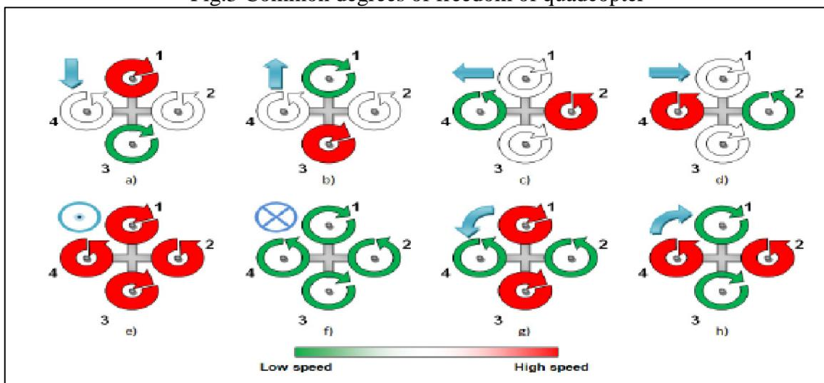
Fig.4 various movements of quadcopter
