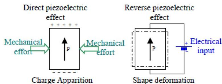
Fig.1 Electromechanical transfer by piezoelectricity
