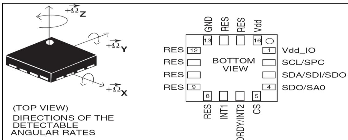
Fig.6 Pin connection of L3GD20
