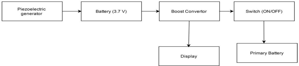
Fig.10 Block diagram for Piezoelectric generator
