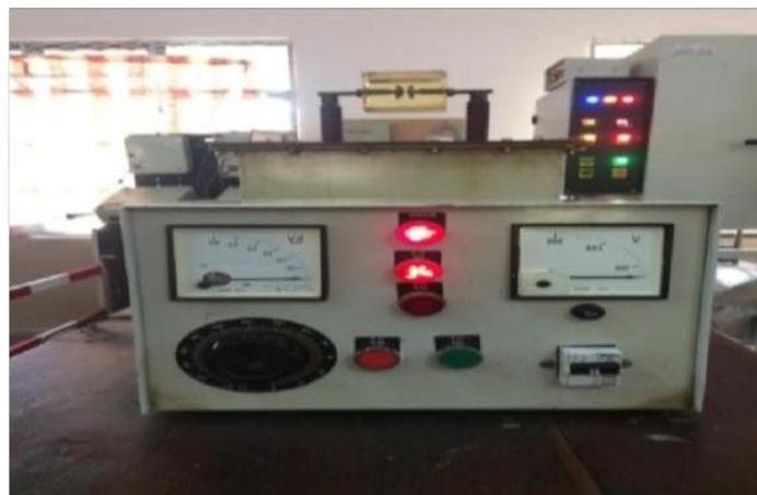
Figure.1.1 BDV measuring apparatus
