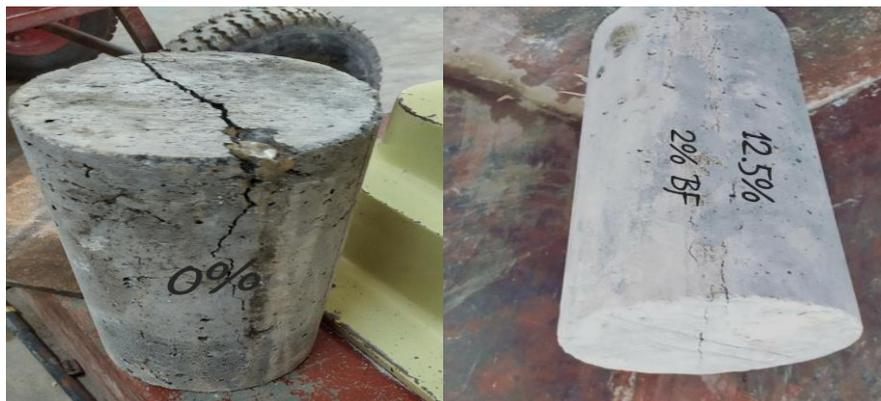
**Figure 3: break safe in split elasticity of cement supplanted with metakaolin**
