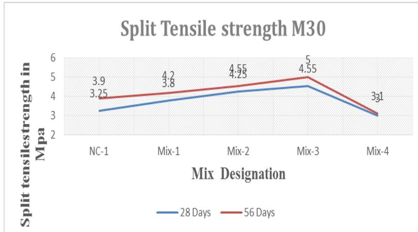
Figure 4: splitting tensile Quality for M30 Grade
