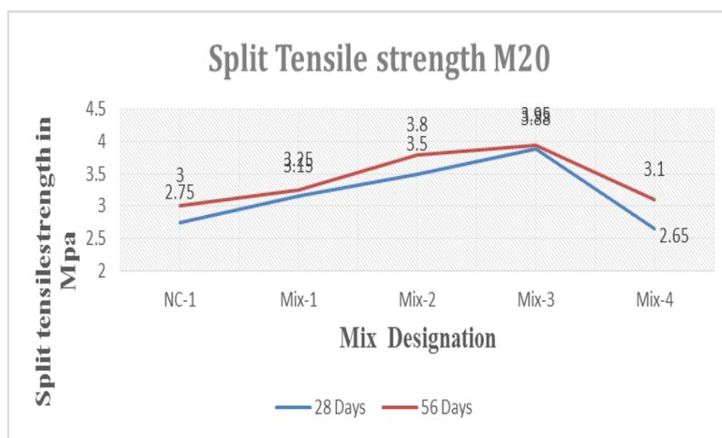
**Figure 3:** splitting tensile Quality for M20 Grade
