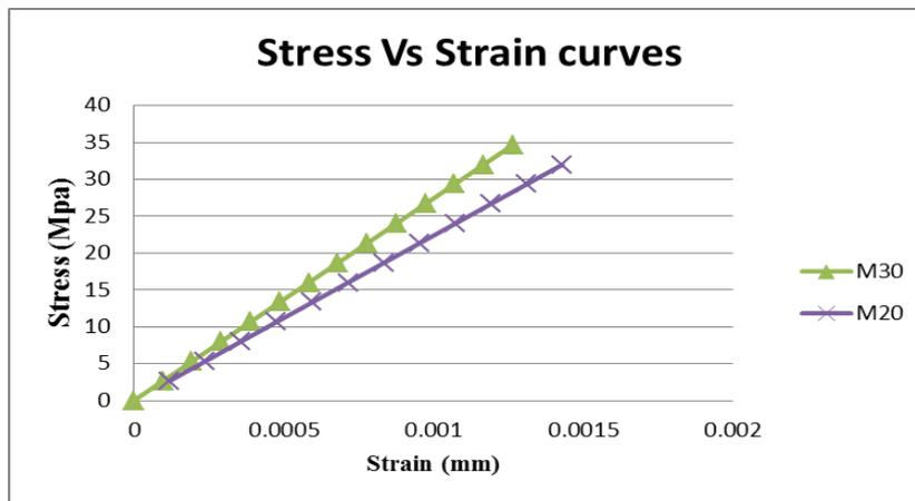
Figure 8: stress – strain plot for RC beams
