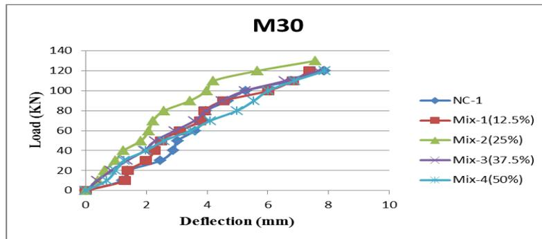
Figure 12: Load Deflection curve for M30
