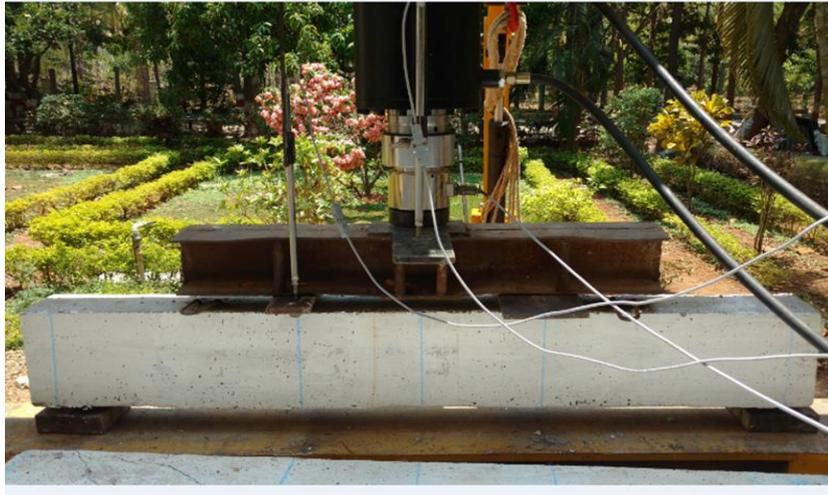
Figure 7: 2-point loading arrangement for RC beams
