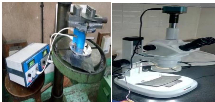
Figure 3: Sensitive drilling machine, dynamometer, fixture for load cell and stereomicroscope
