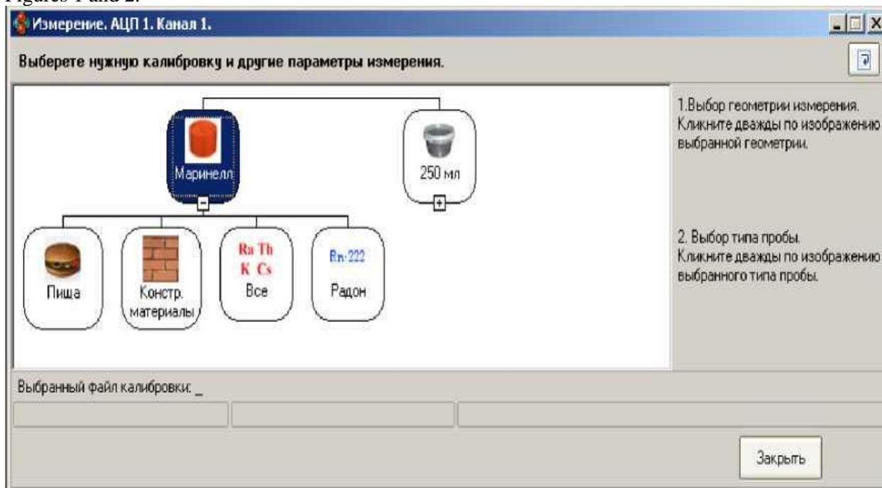
Figure 1. Selection of measurement parameters when calibrating the radiometer MKGB-01 with the "ASW" program.
