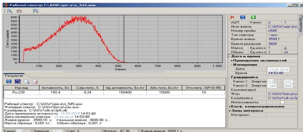
**Figure 3. Calibration data of the MKGB-01 radiometer using the “ASW” program.**
