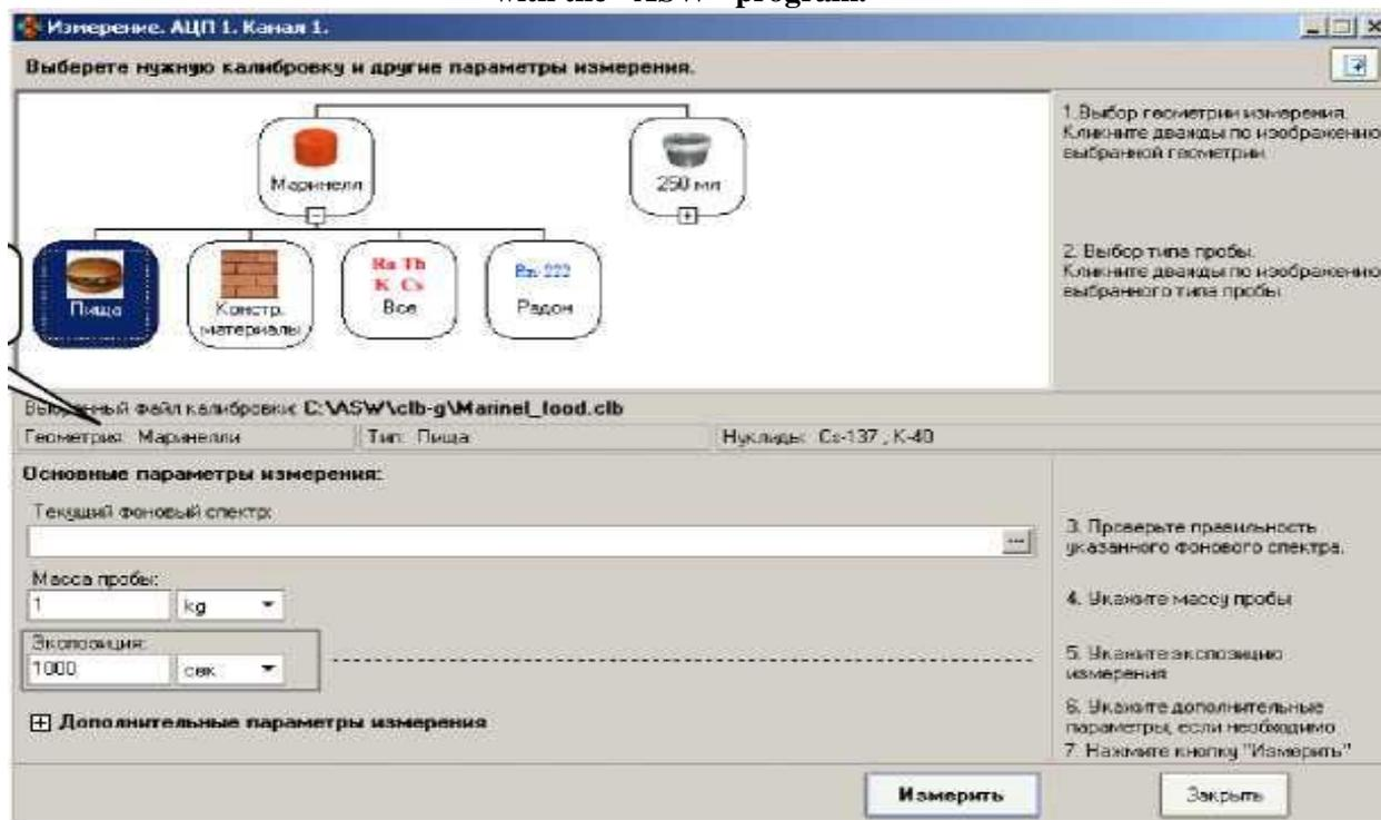
Figure 2. Selecting other measurement parameters: sample mass, spectrum channel, measurement time.
