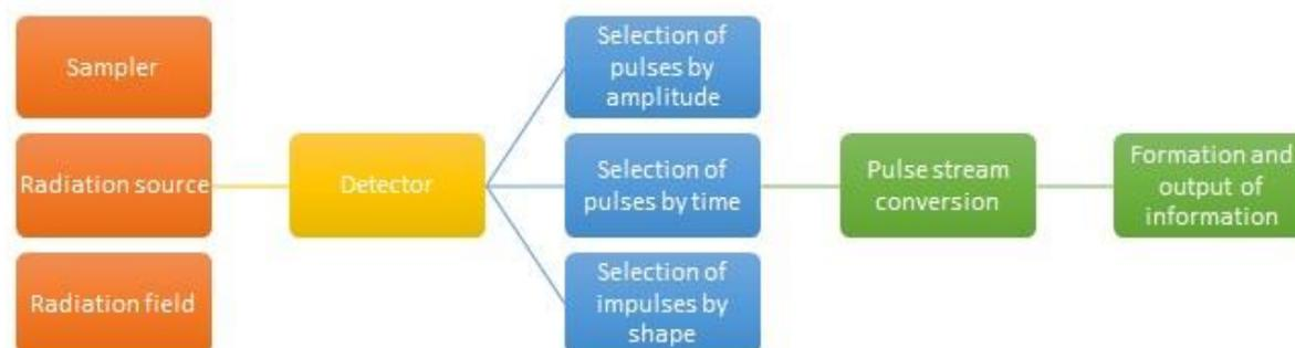
**Figure 1 The general block diagram of most types of radiometers is shown**
