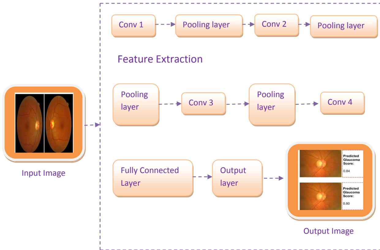
Fig (1.1) Structure diagram for glaucoma prediction using deep CNN algorithm
