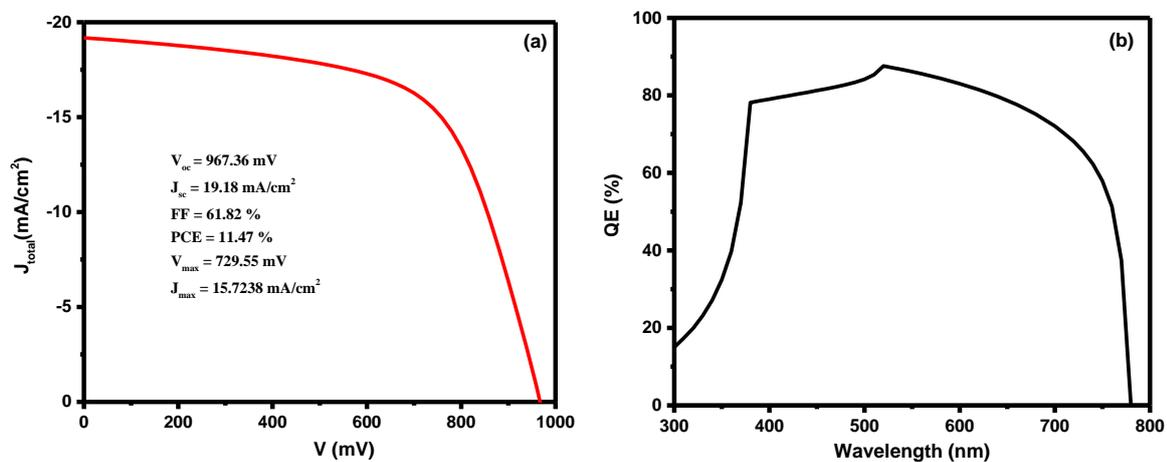
**Fig. 2 Simulated (a) JV characteristics (under light illumination) and (b) quantum efficiency of  $Sb_2S_3$  solar cell.**
