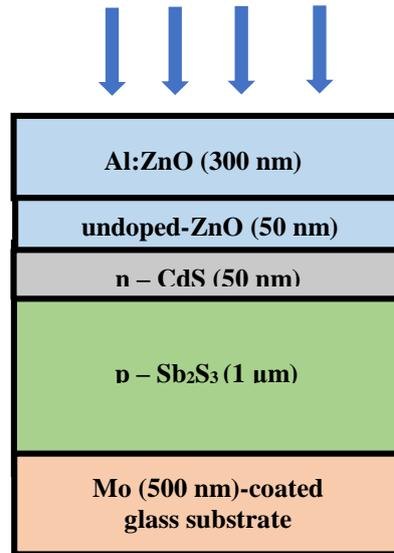
**Fig. 1 Device structure of  $Sb_2S_3$  solar cell.**
