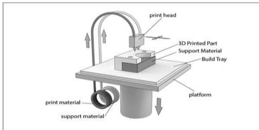
Figure 1 Schematic of FDM process
