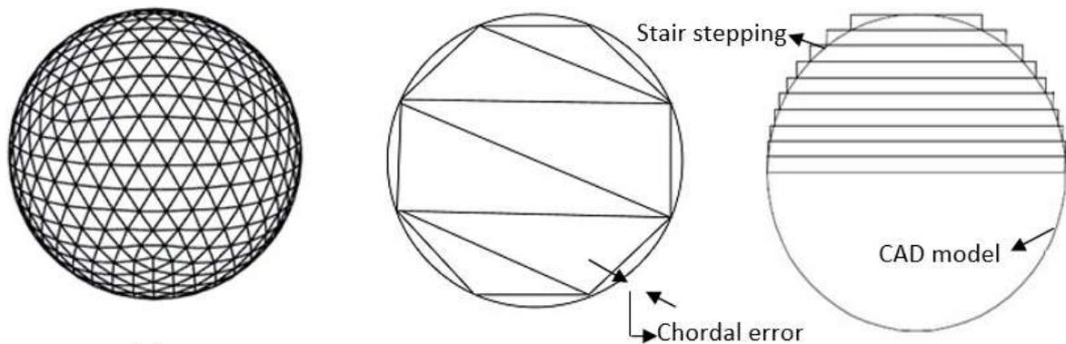
Figure 3 Surface defects produced on FDM parts
