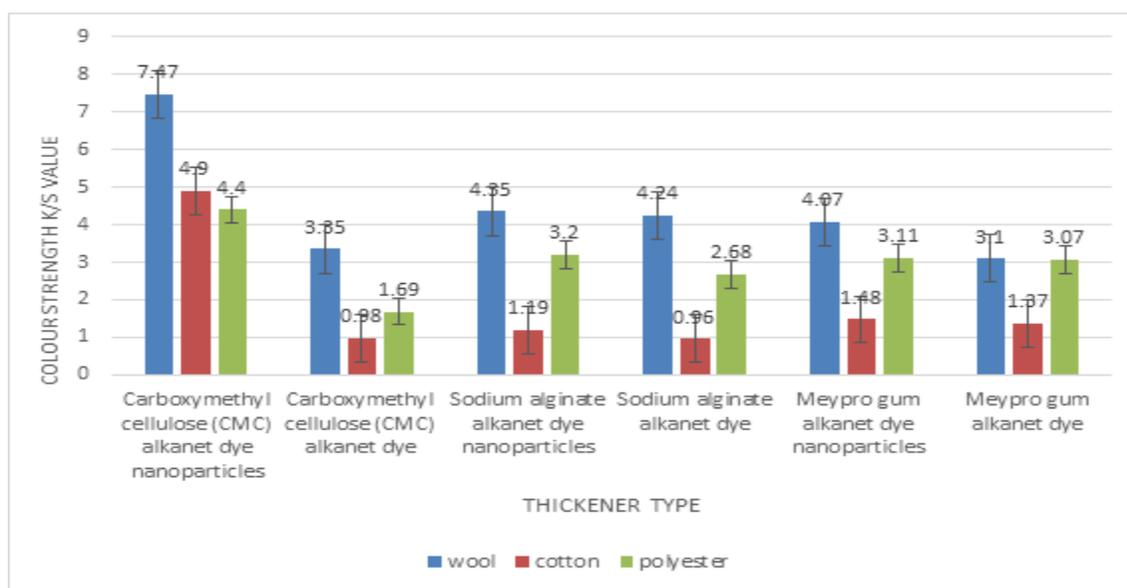
**Fig.4** Effect of thickener type on K/S values of cotton, wool and polyester fabrics printed with alkanet dye and alkanet dye nanoparticles.
