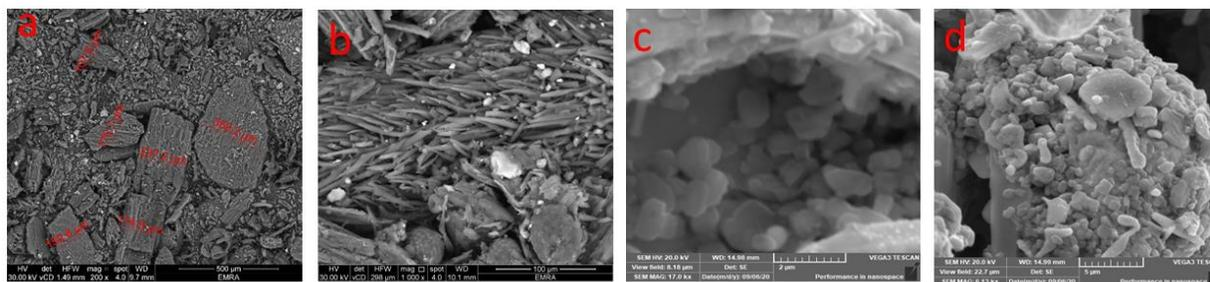
**Fig. 2.** scanning electron microscopy images of alkanet dye (a and b) and alkanet dye nanoparticles (c and d)
