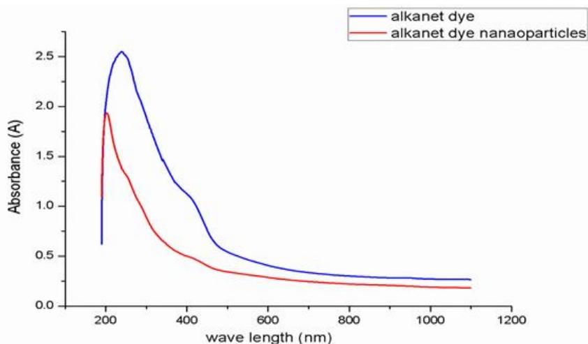
Fig. 1a. UV-vis. spectra of alkanet dye and alkanet dye nanoparticles
