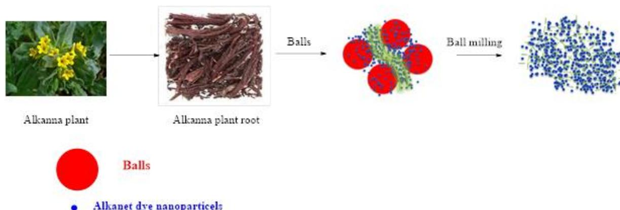
**Scheme 1.** Schematic diagram of alkanet dye nanoparticles production by ball milling
