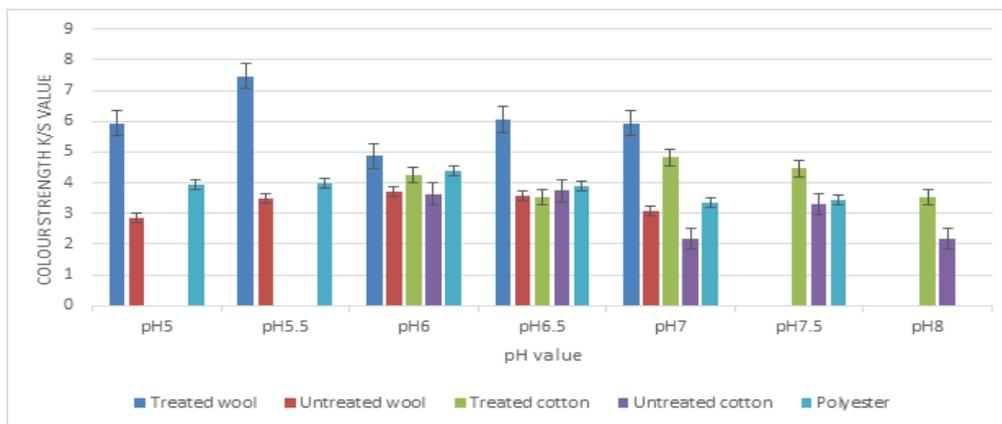
**Fig. 6** Effect of pH value on K/S values of treated and untreated cotton, treated and untreated wool and polyester all fabrics printed with alkanet dye nanoparticles.
