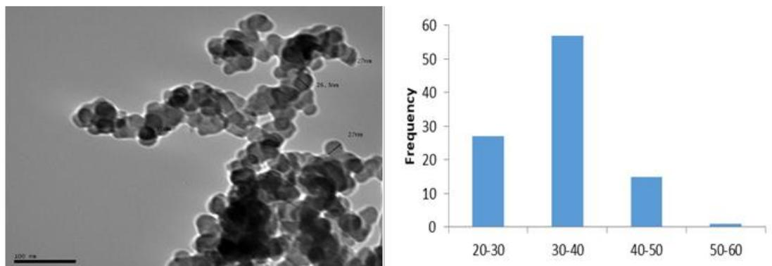
**Fig. 1d.** TEM image of alkanet dye nanoparticles prepared via ball milling and histogram of its nanoparticle size
