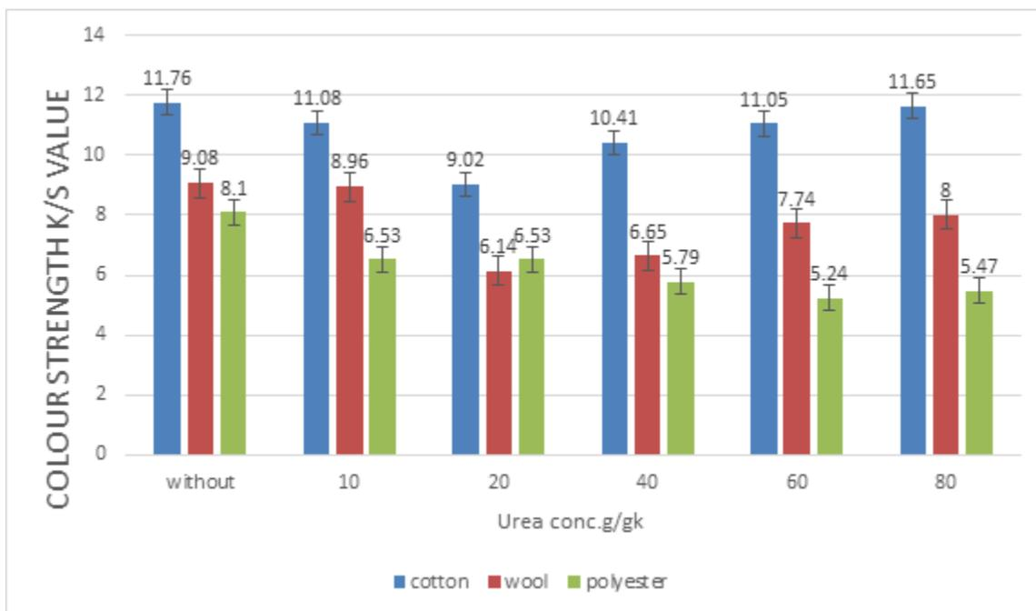
**Fig.8** Effect of urea concentration on K/S values of cotton, wool and polyester all fabrics printed with alkanet dye nanoparticles.
