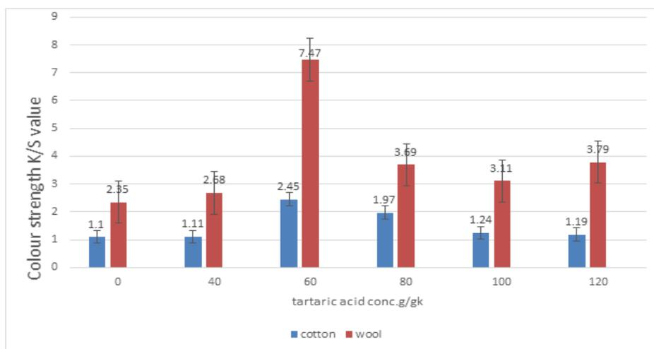
**Fig. 3.** Effect of concentration of mordant on K/S values of wool and cotton fabrics printed with alkanet nanoparticles
