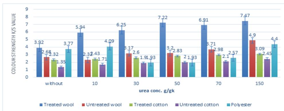
**Fig. 5** Effect of urea concentration on K/S values of treated and untreated cotton, treated and untreated wool and polyester all fabrics printed with alkanet dye nanoparticles.
