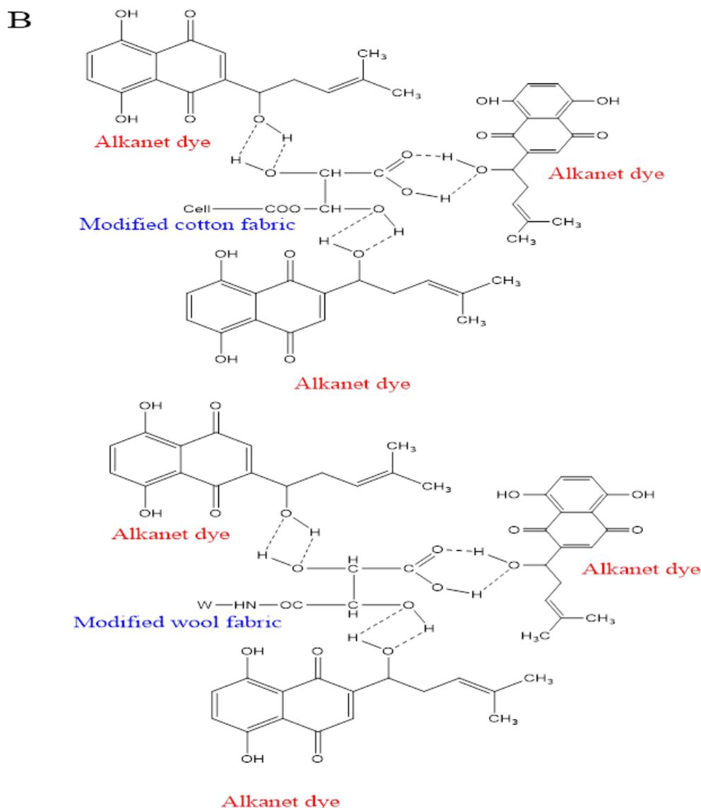
**Scheme 3.** Reaction of alkanet dye with unmodified cotton and wool fabrics (A) and tartaric acid modified cotton and wool fabrics (B)
