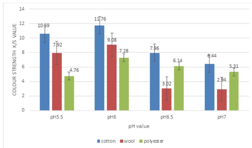
**Fig. 7** Effect of pH value on K/S values of cotton, wool and polyester fabrics printed with alkanet dye nanoparticles.
