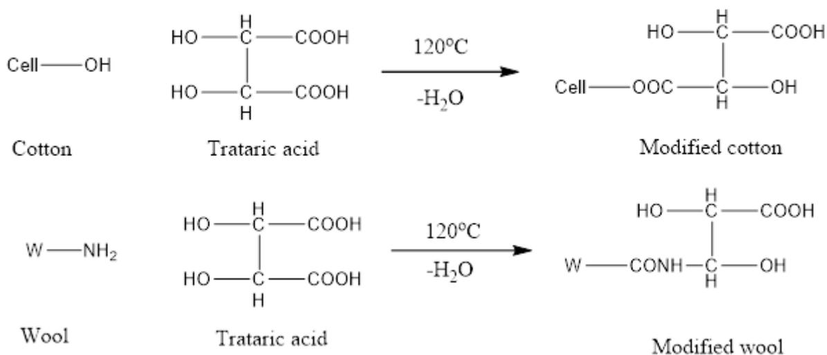
**Scheme 2.** Modification of cotton and wool fabrics via reaction with tartaric acid
