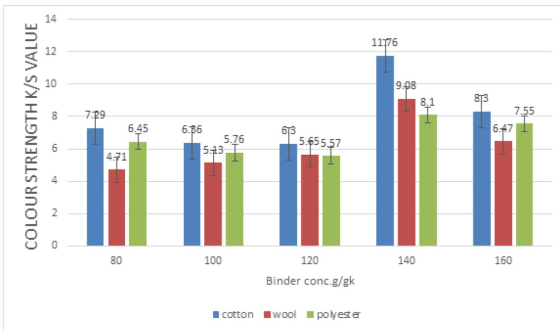
**Fig.9** Effect of binder concentration on K/S values of cotton, wool and polyester fabrics printed with alkanet dye nanoparticles.
