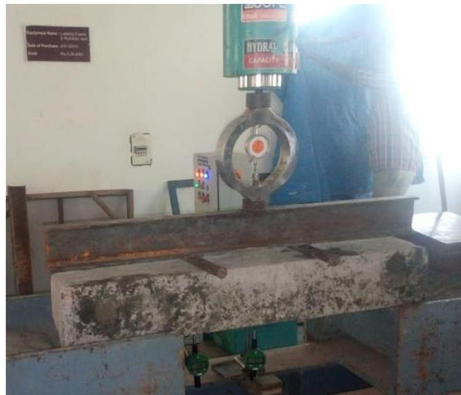
Fig. 3. Flexural Strength Test
