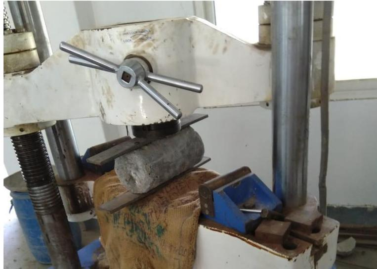
Fig. 2. Indirect Tensile Strength Test
