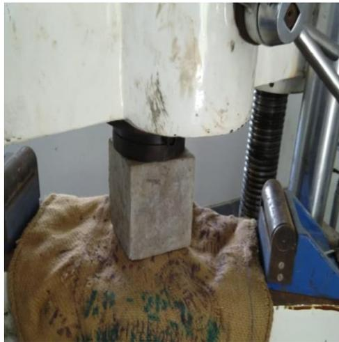
Fig. 1. Compressive Strength Test
