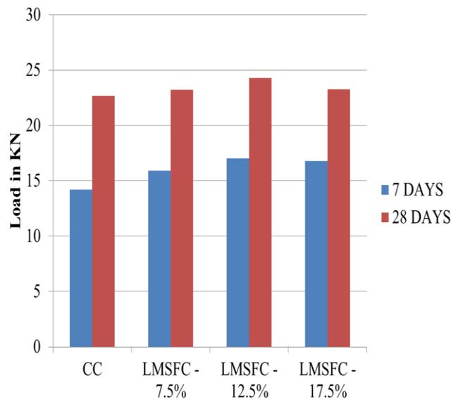
Fig. 4. Compressive Strength Results
