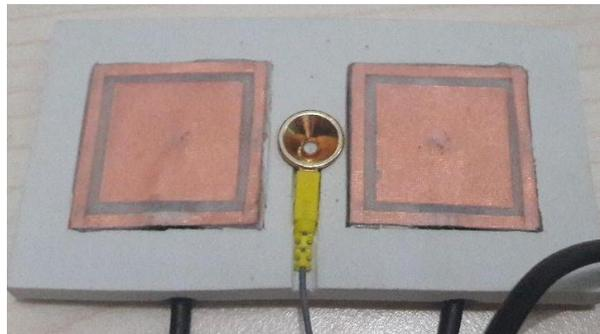
Figure 1. An integrated Brain ECVT and EEG sensor.
