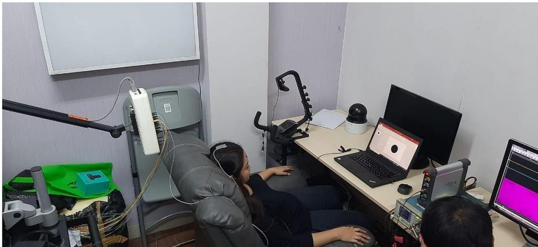
Figure 3. Integrated multichannel EEG-ECVT measurement setup.
