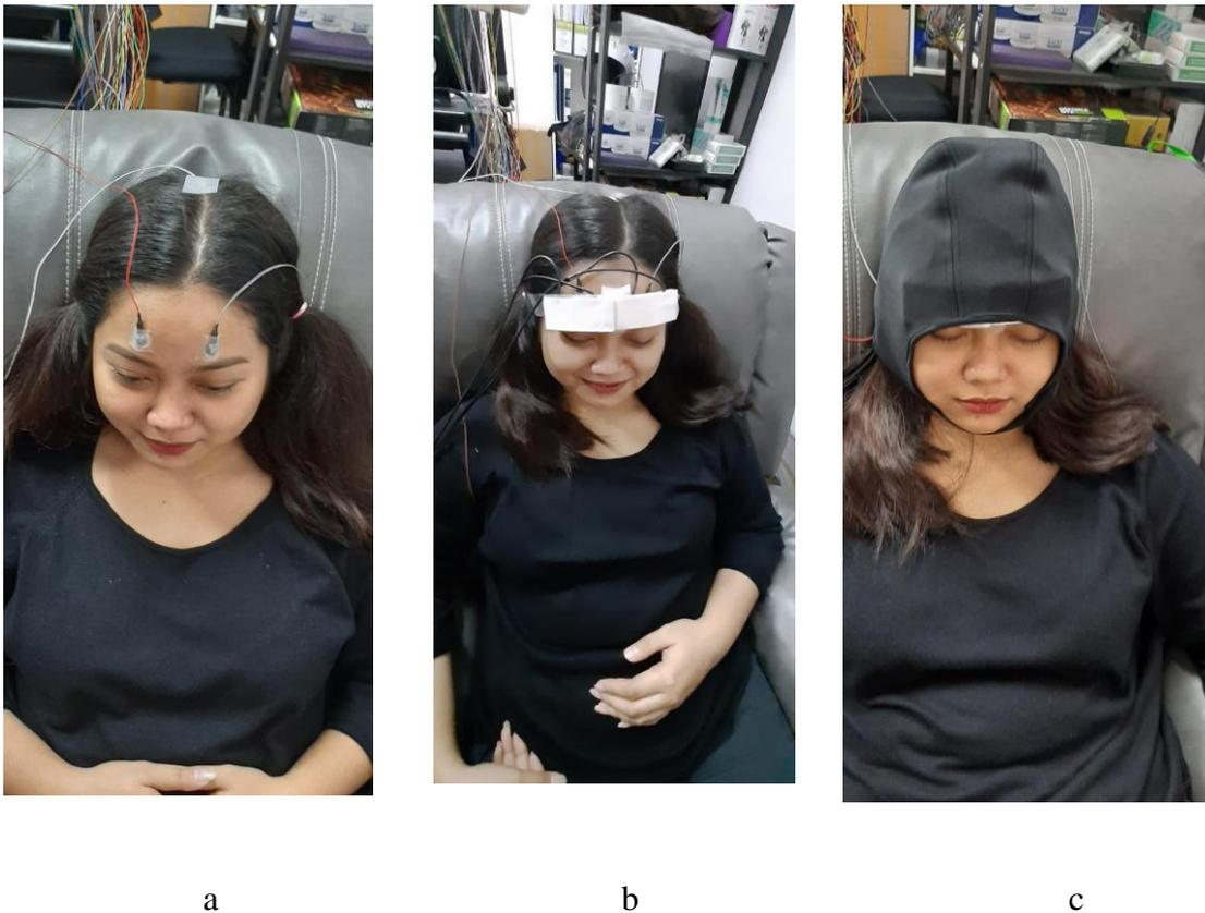
Figure 2. Integrated EEG-ECVT sensor placement on the subject's head.
