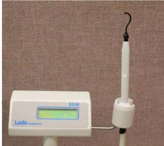
Fig 3- Electrical Caries Monitor (ECM) device (reproduced with permission)<sup>21</sup>
