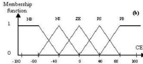
Figure 8. Membership Function for Change in Error E(n).
