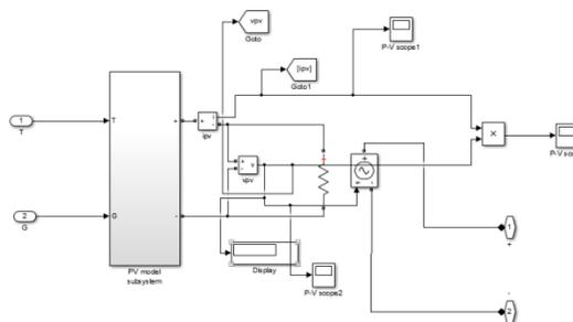
Figure 11. Simulink Model for PV System
