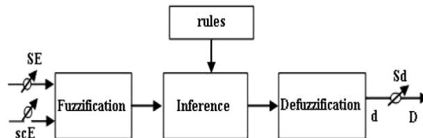
Figure 6. General diagram of a fuzzy controller
