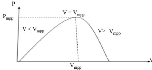
Figure 2. Characteristics of Photovoltaic cell.
