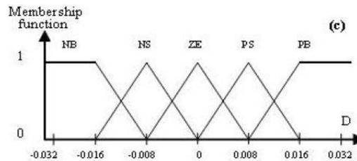
Figure 9. Membership Function for Duty Cycle D(n).
