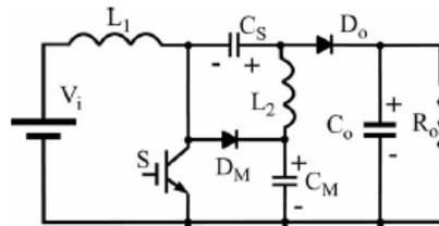
Figure 5. Modified Sepic Converter Circuit.
