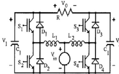
Figure 10. Single phase inverter circuit.
