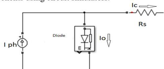
Figure 1. Electrical Model of Photovoltaic Cell.
