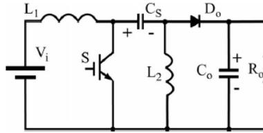
Figure 4. Classical Sepic Converter Circuit.
