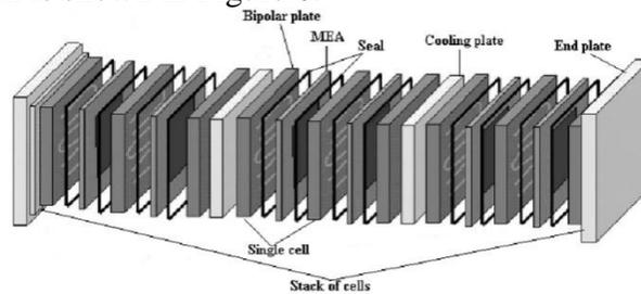
Figure 6 Fuel Cell stack
