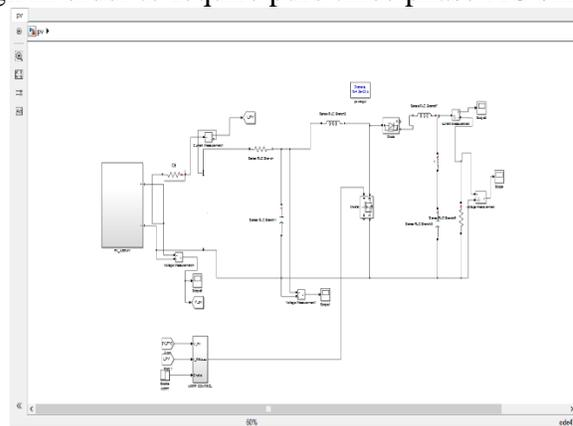
Figure 2 Simulink model of PV array
