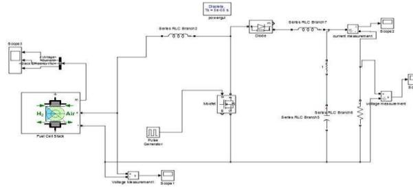
Figure 5 Simulink circuit model of fuel cell stack
