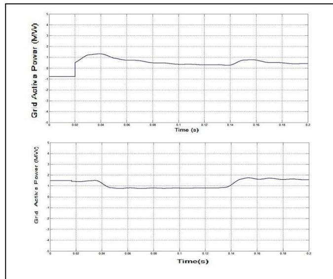
Fig. 11. Grid Active Power without controller and with Controller
