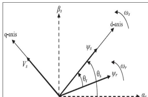
Fig. 3. V and flux vector diagram
