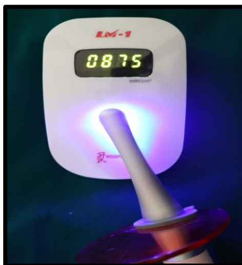
Figure 4: LM-1 LED light meter cure power curing tester
