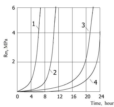
Fig. 1. 1- PC M400, 2- C + 0.1% water repellent on fly ash, 3- C + 0.1% on Gliezha, 4- C + 0.1% on quartz sand.
