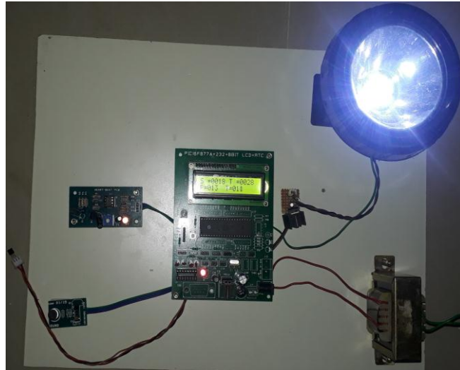
Figure 2.1.2 Working Model Of Transmitter For HMS Using VLC
