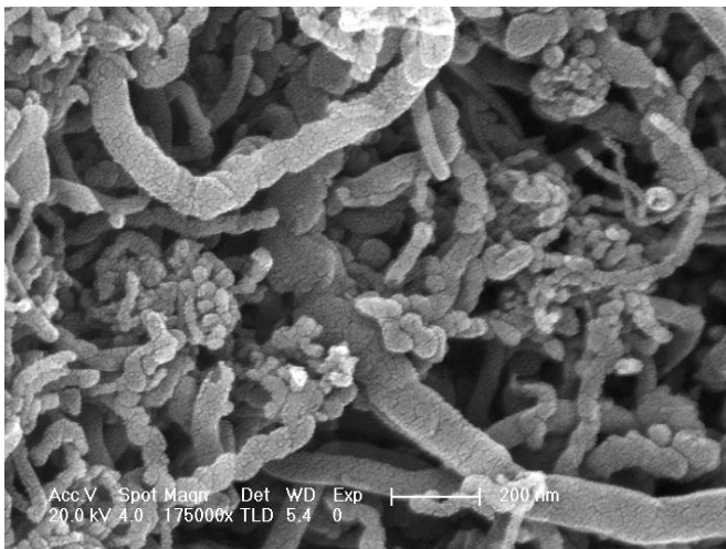
Figure 2a: SEM images of F- MWCNTs – 5-Fu at 200nm
