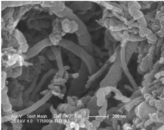
Figure 1a: SEM images of Functionalized MWCNTs at 200 nm
