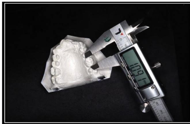
Figure 2: Digital Vernier caliper for measuring mesiodistal dimensions
